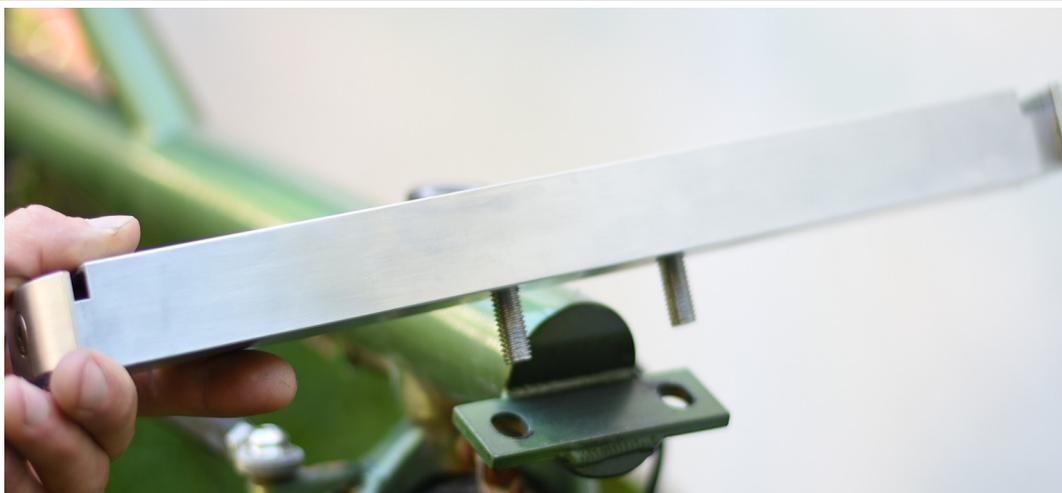
Put the shims and nuts on the screws and tighten them up with 15Nm bis 20Nm.
