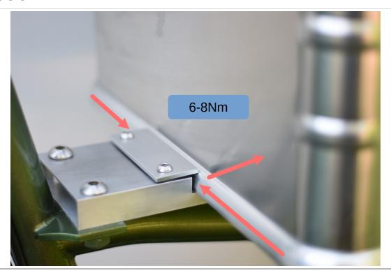
Put the two clamps at the crossbar up and thighten the screws with 6Nm bis 8Nm.
