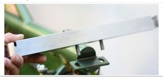
Put the shims and nuts on the screws and thighten them up with 15Nm bis 20Nm.
